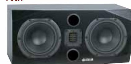
Like the S3A, one woofer acts as a full-range driver with the second woofer joining it only below 150Hz. This effectively doubles the area and power of the woofer when it needs to respond to deeper frequencies, resulting in an exceptional low end without compromising midrange performance. 219443
